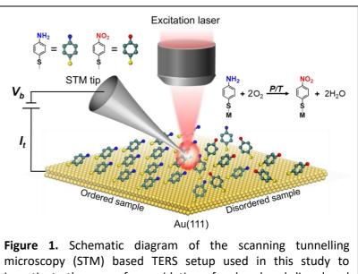
microscopy (STM) based TERS setup used in this study to investigate the on-surface oxidation of ordered and disordered 4-ATP adlayers on Au(111) surface.
